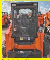
Thanks for the article on my screen guards designed to protect tractor cab windows as well as the tractor operator (Vol. 42, No. 4). I recently built a guard for skid loaders used in the forestry business. The photo shows it mounted on front of a Kubota 95 SVL skid loader.
