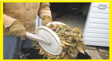
Putting piles of raked leaves into bags is easier with these "leaf paddles" that I made using a couple plastic 5-gal. bucket lids and two pieces of 2 by 2 cut off at about a 20° angle. I used wood screws to attach the pail lids to each angled handle. I rounded off the edges of the wood for a more comfortable grip. Works great! (Larry Floer, Regina, Sask.)
