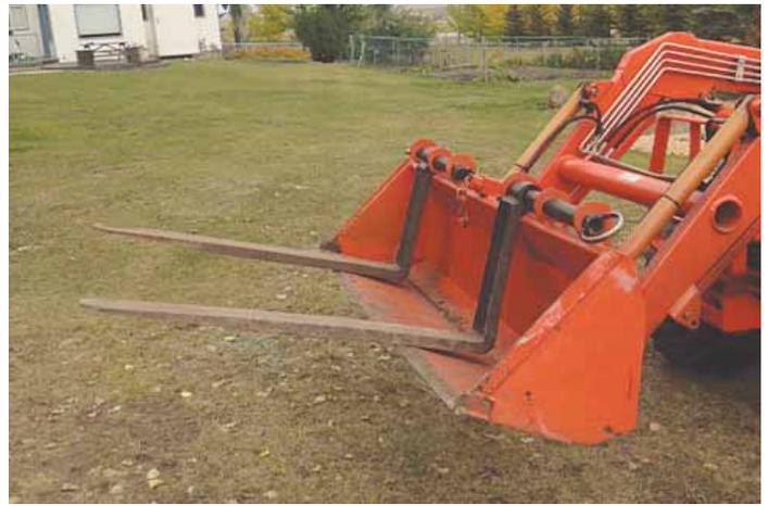
Bucket forklift was made by welding 3 round brackets with holes in them on top edge of bucket, and welding brackets on top of 2 L-shaped forks. Steel rods run through brackets to support forks.
