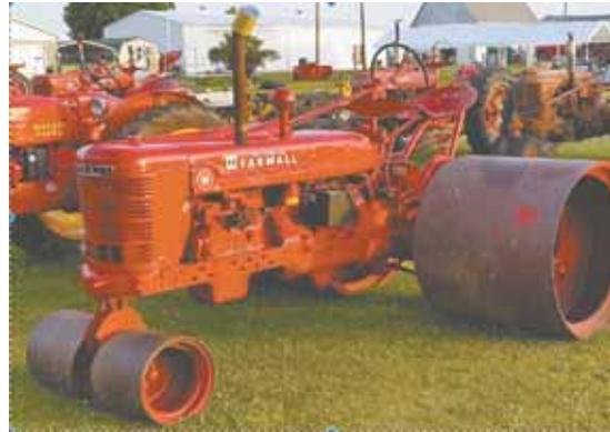
As high as they are wide, the steel wheels on Bill Hedrick's Farmall H were designed to pack sod before it's cut.
