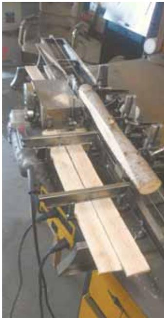
Just 46 in. long, Allan Isaac's 1:12 scale mini sawmill really works. It's powered by an angle grinder motor while a 4 1/2-in. carbide blade does the sawing.
