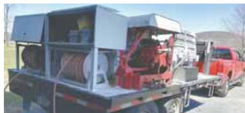
Trailer-mounted whitewashing system includes an air compressor, along with a mixing tank, hoses, tools and accessories. An all-girl team does the work.
