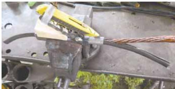
Sid Stubbs uses his bench vise-mounted cable stripper to remove the rubber from battery cables. "I can strip a lot of cables in a very short time," he says.
