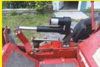
Thanks for the report in your last issue on how a neighbor used an electro-hydraulic cylinder from an old Deere small square bale thrower to automatically raise or lower the deck on my Ferris zero-turn riding mower. The cylinder is wired to the mower battery, so I can use a toggle switch instead of a hard-to-push-down foot pedal to raise or lower the deck.
