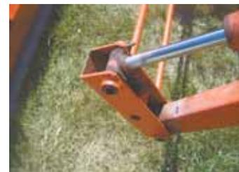
Devine cut the bucket off his tractor's loader arms, then used a combination of tabs and ears to turn the loader and bucket into a versatile quick attach system.
