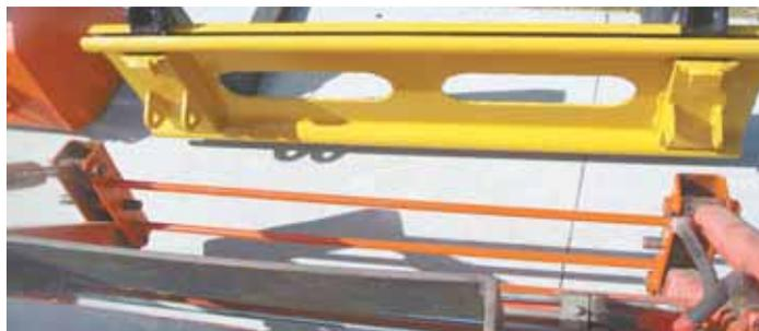
Photo shows how loader arm tabs and bucket ears attach together.
