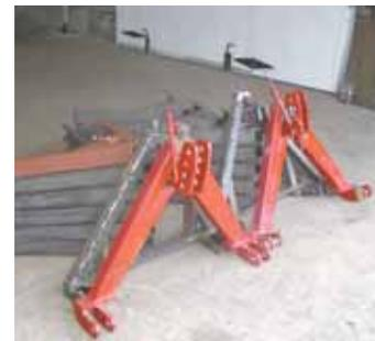
Female hitch is pinned or welded to implement (left) in place of the original 3-pt. connection. Male hitch on tractor installs with a hydraulic cylinder in place of top link.
