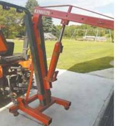
By fitting 3-pt. mounting brackets on a shop engine hoist, Rickie Stich can mount it on back of his Kubota 23 hp. tractor.
