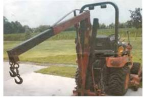
Hoist's hydraulic jack can still be used to control the lifting motion.
