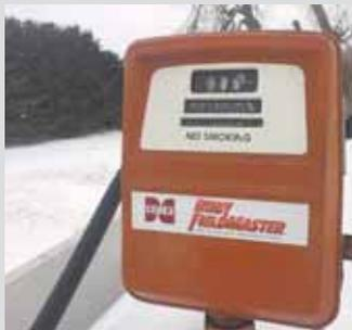
for these pumps, including the brass vanes and the little number wheels that register the gallons dispensed. The impellers and vanes are easy to get at with only 2 bolts holding the cover. I replaced the clear plastic over the dial with a piece I cut out of a clear liter bottle of soda.
