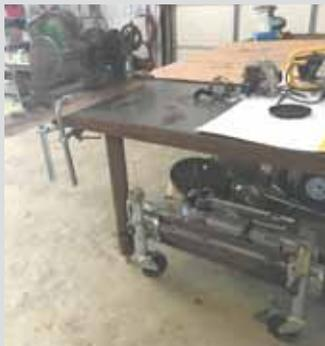
place it in my shop. Putting the table against a wall would limit its use for big projects, and putting it in the middle of the shop would take up too much space. Instead I welded angle irons between the legs on both sides of the table, about 6 in. above a shelf, and then bolted boat trailer jacks onto them.
