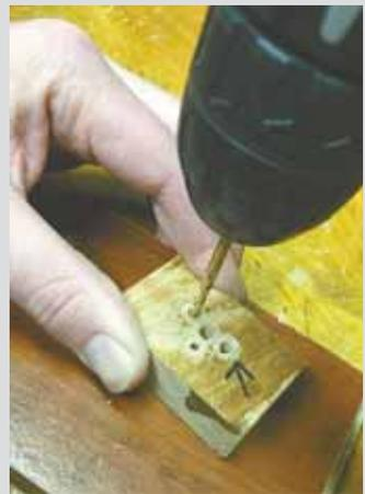
**Ryan Van Der Bill, Sioux Falls, S. Dak.:** "One idea is that when you need to drill a straight hole and you don't trust your eye with a hand drill, take a small block of oak or maple and drill a hole through it with a drill press. Then use that block as a guide when using a hand drill."
