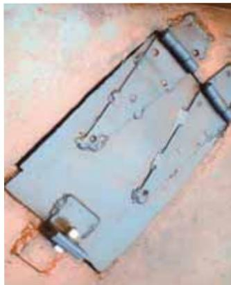
**Fisher cut into the deck on his bush hog mower and installed an 8 by 12-in. hinged access door. "I remove a bolt and flip the door up, then use a grinder to sharpen the blades," he says.**
