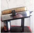
Bacon grease drains out through spout welded into one end of waffle iron, and is collected in a soup can.
