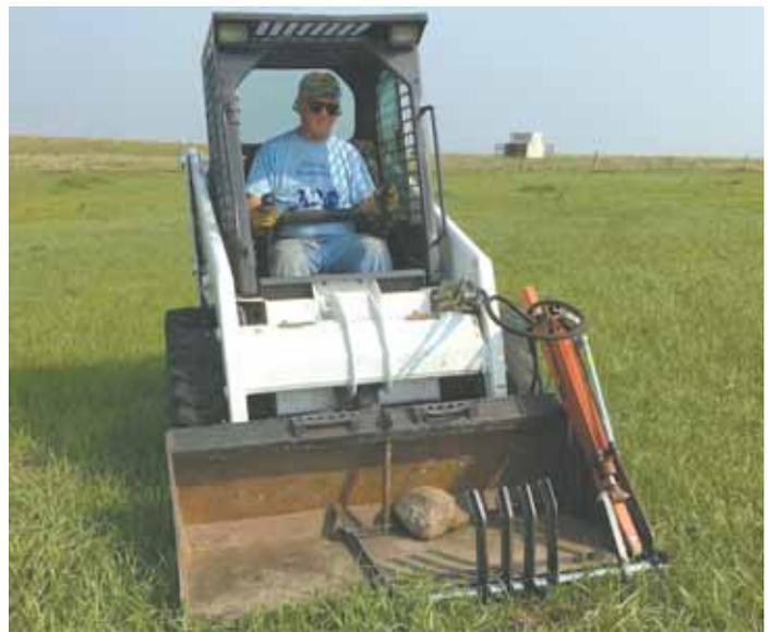
Skid steer attachment uses bucket-mounted rotating forks to load rocks into bucket. It requires no modifications to the bucket or loader.
