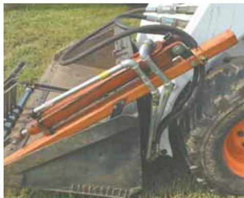
Rock picker teeth are bolted to a short length of pipe that's rotated by a hydraulic cylinder.
