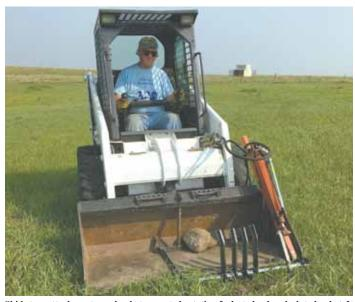
Skid steer attachment uses bucket-mounted rotating forks to load rocks into bucket. It requires no modifications to the bucket or loader.
