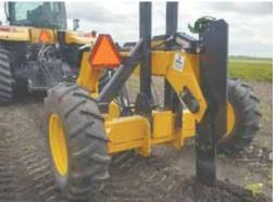
Dave Horn's trailermounted knife cuts through hardpan to a depth of 5 ft., towing a bullet-shaped tunnel maker behind it. Tunnels pull water away from wet spots.
