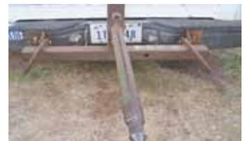
Leer made the bale spear from an old Deere cultivator, adding 2 shorter rods on each side to stabilize the bale.
