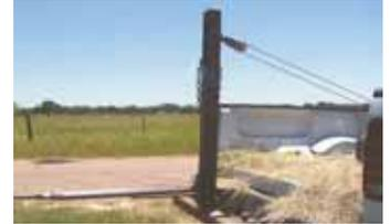
Winch cable goes through pulley at top of carrier’s steel upright.
