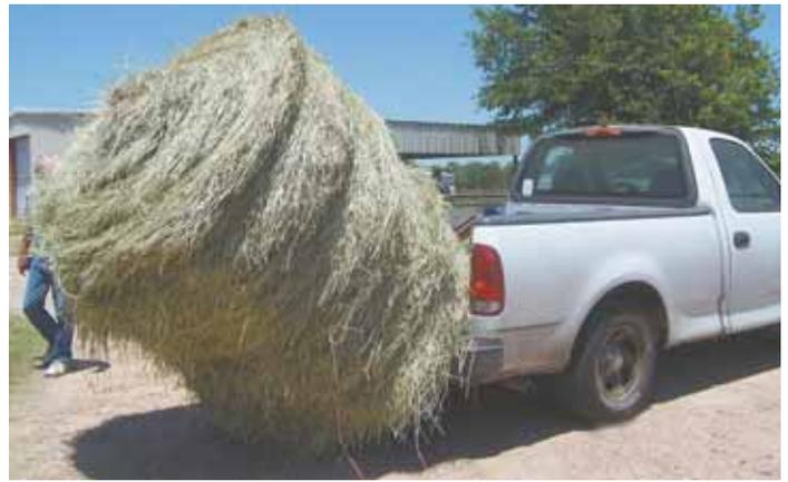
Winch-operated bale carrier mounts on the rear bumper of Bob Leer’s 2004 Ford shortbed pickup. “It’s a fast, efficient way to move round bales,” he says.
