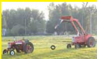
When my dad tried to plow up an alfalfa field with his Farmall Super M in the 1950's, he could not pull his 3-16 plow so he hooked up a Super H to help out. He would hook up two chains with a rubber tire in between to smooth out the pull. It was a "poor man's" substitute for a 4-WD tractor, which did not exist at the time.
