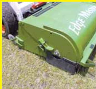
I used to watch city workers with rakes and shovels cleaning the edges along sidewalks and then running a sweeper over them. I figured there had to be a better way so I built my new skid loader-mounted Edge Master power sweeper, which is designed to edge and sweep in a single pass. It can clean and edge 100 ft. of sidewalk in less than 2 min.
