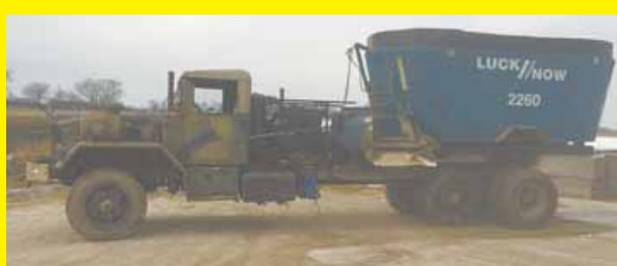
A few years ago you ran an article about the self-propelled, side unloading feed mixer I built by combining parts from a military semi tractor and a pull-type feed mixer (Vol. 35, No. 2). The mixer is made entirely from used equipment, and any parts like chains or sprockets were all purchased online at surplus prices.
