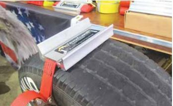
Steel traction claws strap to vehicle's drive tires to free stuck vehicles.
