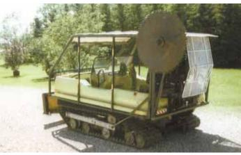
Big 32-in. dia. sawmill blade mounts 6 ft. off the ground alongside ATV's rollbar. As Nielsen drives along, bent-over small trees are cut by blade.
