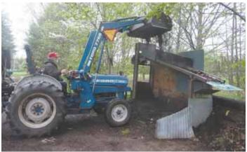
Rod Stremlo's big home-built sifter is able to handle compost using a front-end loader. There's room underneath for loader to retrieve a bucketful of sifted compost.
