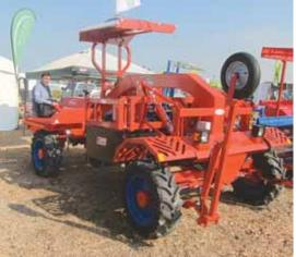
Designed mainly for vegetable crops, Scorpion self-propelled automatic weeder can remove weeds between the rows and also between plants in the row.
