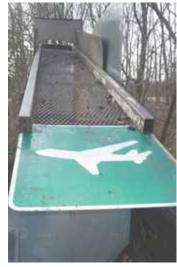
The 2-ft. wide by 12-ft. long sifter mounts on a frame made from old goal posts and steel tubing.
