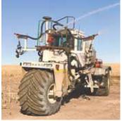
Sprayer carries 3 tanks including a large 1,600-gal. tank and two 50-gal. tanks.
