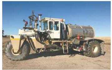
Marvin May converted a Mertz self-propelled floatation sprayer into this "Fire Buggy". Fire nozzles on each side are controlled by linear actuators.
