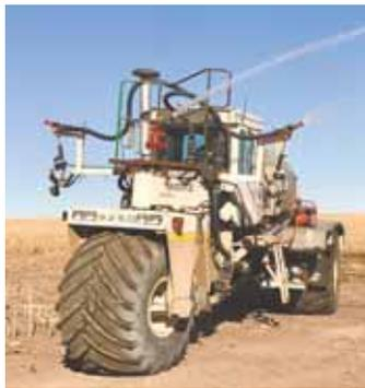
Sprayer carries 3 tanks including a large 1,600-gal. tank and two 50-gal. tanks.
