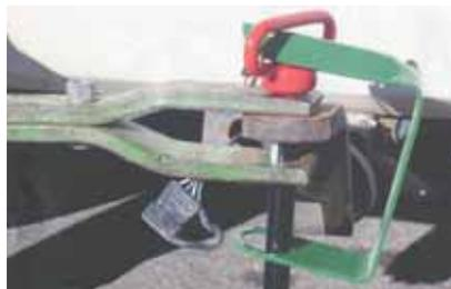
Safety hitch pin bracket comes with a small hole on top to insert a snap ring, and a 1 1/2-in. dia. hole at bottom for the pin.
