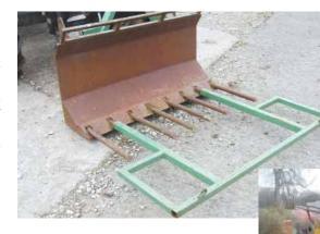
Alistair Robert used 2-in. box tubing to build this loadermounted ATV hauler. The frame slips over 2 forks on loader bucket.
