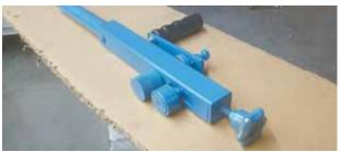
Hand-cranked roller consists of a 1-in. sq. steel tube with 2 steel rollers. rim." Contact: FARM SHOW Fo
