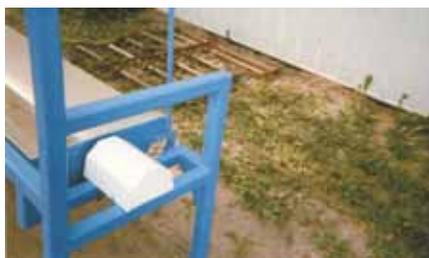
Operator releases a latch at one end of trough and grabs a metal rod to tip trough forward. It automatically relatches when tipped back into place.
