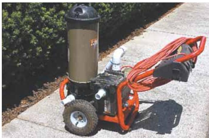
Browning mounted the pump and canister filter off a commercial swimming pool cleaner on the frame of an old pressure washer. “The pool cleaner’s big 10-micron filter removes most of the impurities in the water,” he says.
