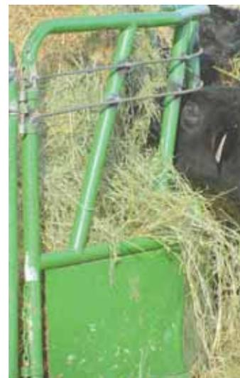
To keep calves from climbing into his big bale feeder, Thomas welded a pair of 3/8-in. rebars across each stanchion, just below the feeder’s top rail.
