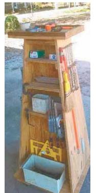
Cabinet sides taper from 22-in. edges at the bottom to 10-in. edges at the top. The taper makes cabinet hard to tip.
