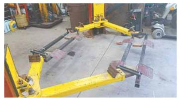
Twin sets of wheel support rails are attached between the lift arms of hydraulic, 2-post car lift, making it easy for Brauer to work on his garden tractors.
