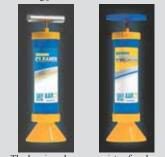
The bearing cleaner consists of a plunger inside a cylinder-shaped chamber; a screwon, cone-shaped plastic base; and a small black cone. The operator fills chamber at least 3 in. deep with cleaning solvent. He then places the cone over the bearing and pushes down on the plunger to flush all the grease out of the bearing. At the same time, the cleaning solvent will be forced up through the bearing's rollers.
