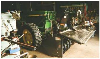
Hinged, hydraulic-operated "door" on front of snowblower is raised up or down by pulling a lever in the cab. With door all the way down Krueger can push slush around without getting it into the auger. To use the snowblower again he just raises the door.
