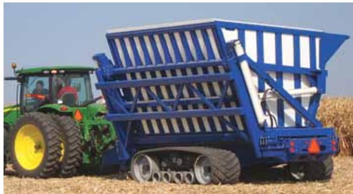
Side dump grain cart is equipped with 4 large hydraulic cylinders – 2 to raise and lower the box and 2 to tilt and dump it. There’s no pto, augers or fighting to wear out.
