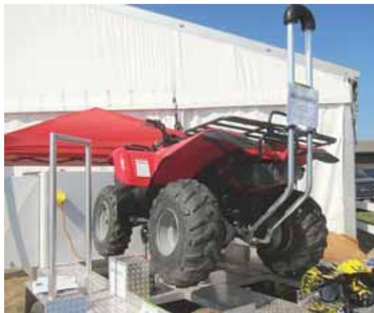
The rounded shape and padding at the top of the Quadbar reduces potential injury, and also allows the point of contact to slide along the ground instead of digging into it.
