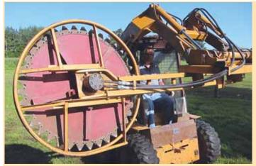
Giant cutter wheel uses mower sickle sections bolted around the perimeter of a 36-in. dia. steel plate to clear a 42-in. wide path. Plate is shaft-driven by a hydraulic motor. **Giant Cutter Wheel Cleans Up Fence Lines, Trims Trees**
