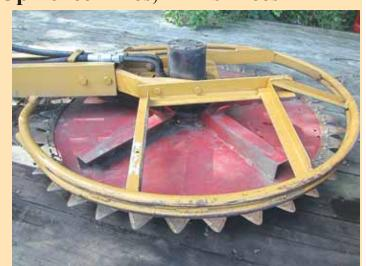
A metal guard made from round tubing lets Majerus cut up close to fence posts without damaging the blades.
