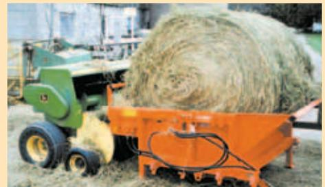
**Machine unwinds bale directly over pickup reel of any small square baler. Here, a 5-ft. wide, 6-ft. dia. bale weighing about 1,200 lbs. is being unwound into a Deere 336.**
