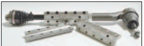
quires no special tools or skills. Simply place the two halves over the tie rod and line up the machined holes. Insert and tighten the 10 allen head bolts and snug down the smaller set screws to keep the sleeve from moving around.
