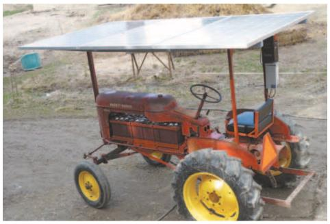
Drew Gailius converted this old Massey Harris tractor from gas to solar, replacing the engine with a 48-volt DC motor and transmission. Three 250-watt solar panels mount horizontally on an overhead frame.
