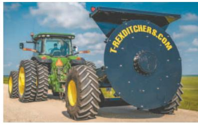
With its 8-ft. spinning wheel, the **T-Rex Rotary Ditcher moves** up to 10 times more dirt than pull-type scrapers, backhoes and dozers. And, it throws dirt evenly over a 300ft. distance without leaving big piles.
