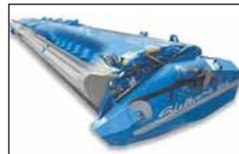
upward. As the combine moves through the field, the fingers strip grain heads and some of the straw from the standing crop and deposit it onto a conventional auger that moves it to the feederhouse.
