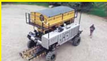
“Power Unit” Self-Propels Grain Drill
