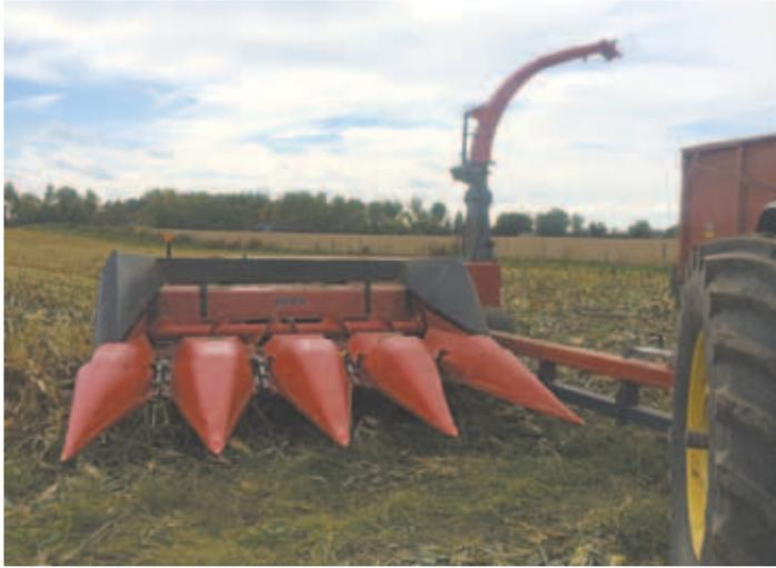
Marvin Bearinger's cob meal harvester was made from several different components, including the cutterhead off a Deere 3960 pull-type silage chopper, a Case IH cornhead, and the feederhouse off a Case IH combine.
