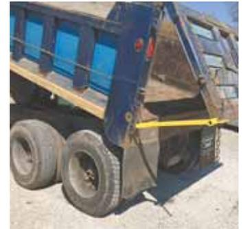
**Dump bed locks, left, hold truck bed securely in the “up” position. At right, Gate-Lok safety bar secures a truck endgate in the open position.**
