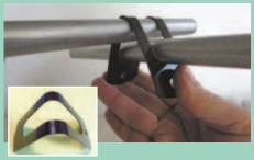
To use the clip you squeeze both ends and slip in pieces of conduit, and then release. Spring tension holds conduit tightly in place.
