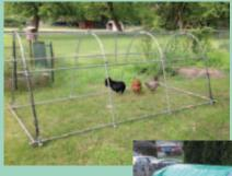
Clip was originally designed to create trellises and low tunnels for gardening, but can also be used to make other types of structures. Specially designed spring clip is used as a fastener for 1/2-in. metal conduit, allowing you to put up greenhouses and storage sheds without using tools.
