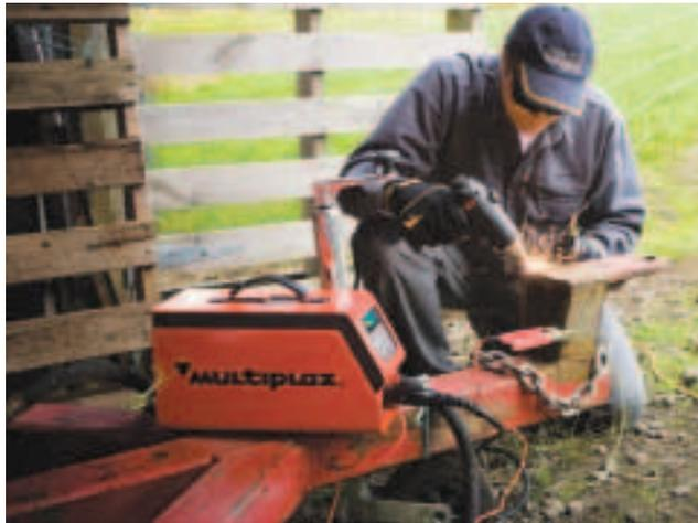
**Not much bigger than an old-time radio, all the Multiplaz 3500 welder needs is 110 or 220-volt current, water and alcohol.**
