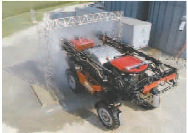
Neil Welsh keeps his self-propelled sprayer clean with this drive-through equipment washer. Pipe framework bolts to large concrete slabs on either side.
