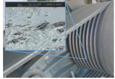
Photo shows a pulley treated with Vulcan Grip on a Claas 980 self-propelled forage harvester. Vulcan Grip's ultra-hard microtexture (inset) resembles an asphalt road surface under a microscope. The treatment reportedly increases V-belt grip and doesn't wear out.
