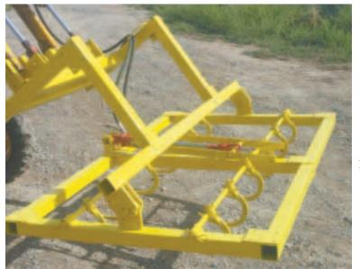
Kornkven also built this bale grapple to handle up to 4 bales at a time. It was featured in FARM SHOW'S Vol. 40, No. 1. Home-built bale accumulator, (on right) rides on wheels that go between the furrows on flood-irrigated hay fields.
