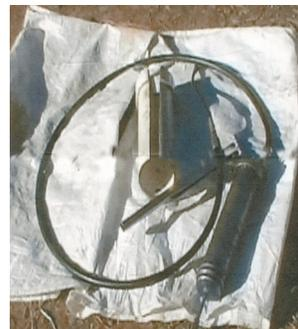
Tom Lass carries his 5-ft. long grease gun hose extension in a homemade holster, made from 3-in. dia. pvc pipe, that hangs from his belt.
