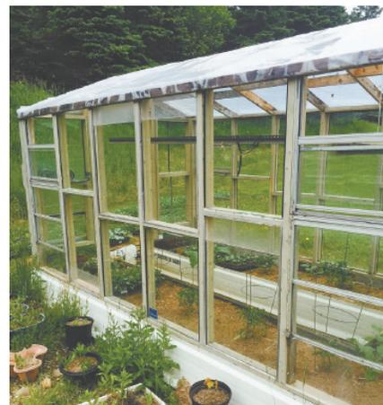
Harry Coates cut off the back half of a 72-passenger bus, removed the floor and used windows from front half of bus to give his greenhouse two sets of windows down each side.
