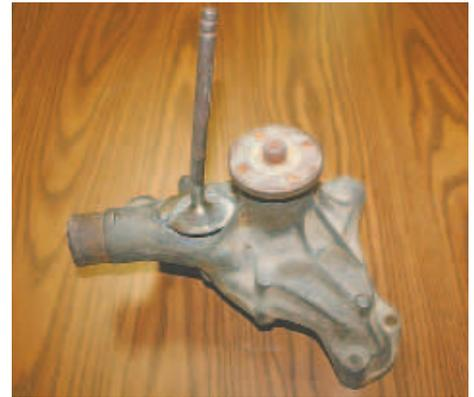
**Magna 777 rod provides machinable welds that won't crack on most types of cast iron. Photo shows a steel valve welded to a cast iron pump.**
