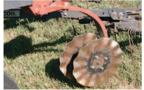
**Coultter kit includes 18-in., 13-wave boron earthen hardened coultter blades. Kit is now fitted with 4 bearings to make it even more heavy-duty. Works in wheat stubble and corn stalks.**
