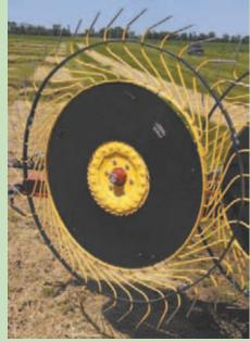
Silencer consists of 1-piece plastic bands that slip over rake wheel teeth and bolt together on the ends. Bands reduce damage to teeth in rough conditions.
