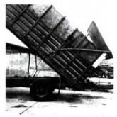
angle iron that runs around the outside of the truck bed in order to run the cable directly down to the truck frame. He welded a short piece of 3/4-in. pipe into the hole to thread the cable through.
