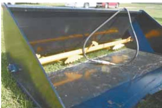
MAC Bucket is designed with a beater bar to chew up manure. Works great for spreading mulch on gardens or litter in poultry facilities.
