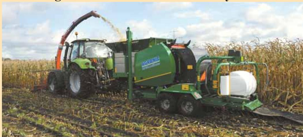
Towed through the field by a forage harvester blowing silage into the hopper, Agronic silage baler compresses and then drops plastic-wrapped bales out the back.
