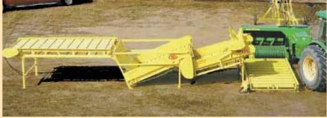
Simpson recently introduced a four piece machine. While one bale is being unrolled for rebaling, you can load another bale onto the prep-table. When the first bale is done, you just flip a lever to advance another roll into the unroller chamber. (Unit shown is four piece model.)
