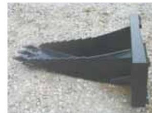
Skid loader-mounted stump bucket is fitted with teeth and serrated sides that tear out roots.
