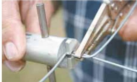
Using the Wire Splicer requires an overlap of about 6 in. of wire, and a needle-nosed vicegrip to hold the wire tight during splicing.
